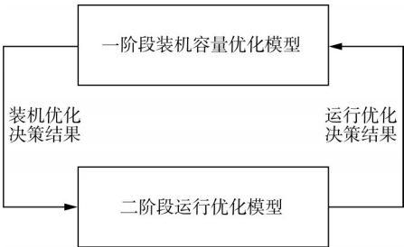
图2 两阶段鲁棒模型迭代求解示意图 Fig. 2 Sketch diagram of iterative solution process for two-stage robust optimization problems
