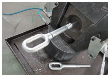
(c) 钢锚与钢芯压接
