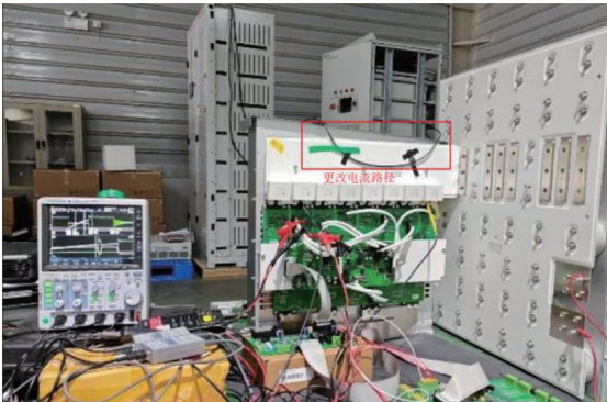
图 8 电流路径更改后实物图 Fig. 8 Physical diagram after changing the current path
